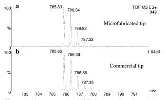
**Figure 3.** Mass spectra of 1  $\mu$ M GFP B obtained from (a) a singlenozzle emitter (10  $\mu$ m  $\times$  8  $\mu$ m) and (b) a commercial capillary tip (i.d.  $\sim$ 10  $\mu$ m). Voltages of 4.5 and 2.1 kV were applied to the fabricated emitters and the commercial tips, respectively. The flow rate was 0.6  $\mu$ L/min for all tips.
