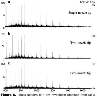
**Figure 5.** Mass spectra of 1  $\mu$ M myoglobin obtained from (a) a single-nozzle emitter, (b) a two-nozzle emitter, and (c) a five-nozzle emitter.
