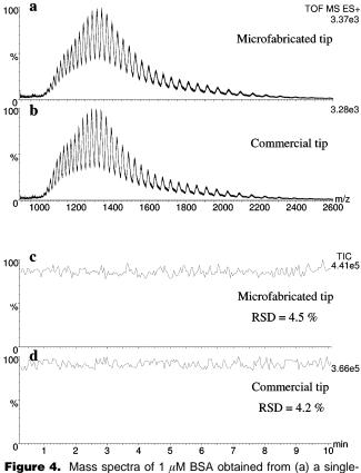
**Figure 4.** Mass spectra of 1  $\mu$ M BSA obtained from (a) a singlenozzle emitter and (b) a commercial tip. Total ion counts of 1  $\mu$ M BSA over time obtained from (c) the single-nozzle emitter and (d) the commercial tip. The RSD was 4.5 and 4.2%, respectively.
