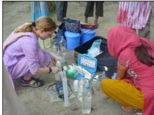
Photo: Kristin Kowolik (left) and Mahbuba Iasmin Ahmed (right) measure water parameters (pH, DO, and arsenic concentration) at a tubewell in Besgao. Photo credit: Shefah Qazi (June 2008)
