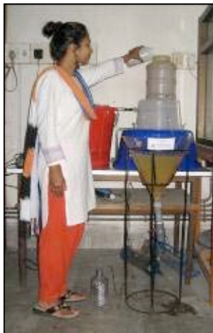
Photo: Shefah Qazi tests the small-scale prototype clarifier in the BUET laboratory. Photo credit: Johanna Mathieu (June 2008)
