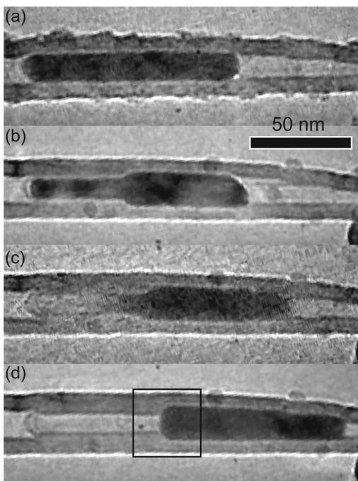
FIG. 2. A time sequence of TEM video images showing the controlled movement of a cobalt catalyst particle.
