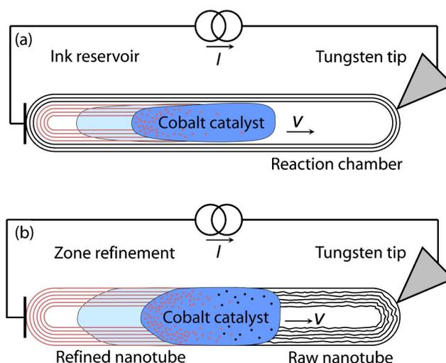
FIG. 1. (Color online). Schematic diagrams of the two modes of operation. (a) The ink reservoir method. As the catalyst moves, carbon initially dissolved in the catalyst particle (the “ink”) precipitates out and forms a new high-quality CNT (red). (b) The zone refinement method. The catalyst particle continuously refines the raw, defective nanotube on the right (black) into a higher-quality nanotube on the left (red).
