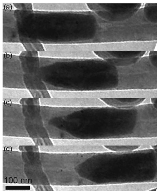
FIG. 4. A time sequence of TEM video images showing a cobalt catalyst particle cannibalize a raw nanotube to its right and reform a CNT to its left as it moves toward the anode.
