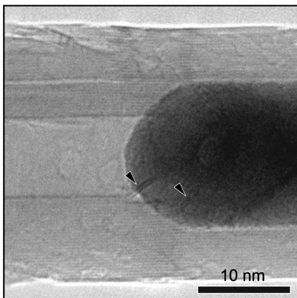
FIG. 3. TEM micrograph of a high-quality multiwall CNT growing within the core of a larger nanotube reaction chamber. This is the area outlined in Fig. 2(d). The image clearly shows the formation of a new, high-quality 11-wall CNT streaming from the end of the catalyst particle. Arrows mark multiple double graphene sheets emerging from the catalyst.
