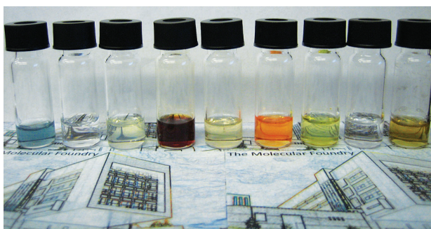
Figure 5. Dispersions of \text{BF}_4^-/\text{DMF} passivated nanocrystals. From left to right: ITO, AZO, \text{TiO}_2 , \alpha\text{-Fe}_2\text{O}_3 , CdSe/ZnS ( \lambda_{\text{em}} = 545 \text{ nm} ), CdSe/ZnS ( \lambda_{\text{em}} = 605 \text{ nm} ), CdSe/CdS quantum dot/quantum rods ( \lambda_{\text{em}} = 619 \text{ nm} ), upconverting \text{NaYF}_4:\text{Yb/Tm} , and Ag nanocrystals.
