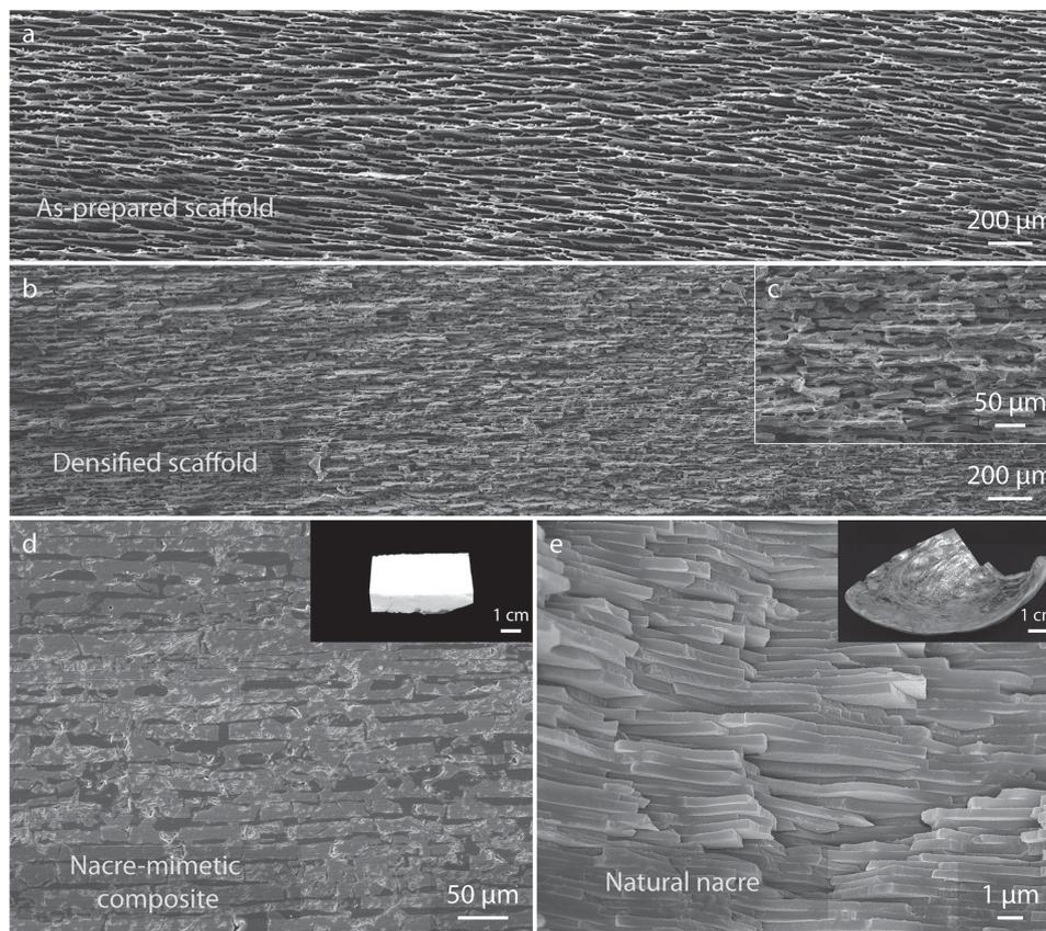
**Figure 2.** Structure of nacre-mimetic HA/PMMA composite compared to natural nacre. SEM images of a) HA scaffold prepared by bidirectional freezing, and b,c) densified scaffold by uniaxial pressing. d) HA/PMMA composite fabricated by bidirectional freezing and in situ polymerization shows a similar “brick-and-mortar” structure as e) in natural nacre. (Note that the images in (d) and (e) are intended to highlight similarities in structure, but have somewhat different magnifications.)
