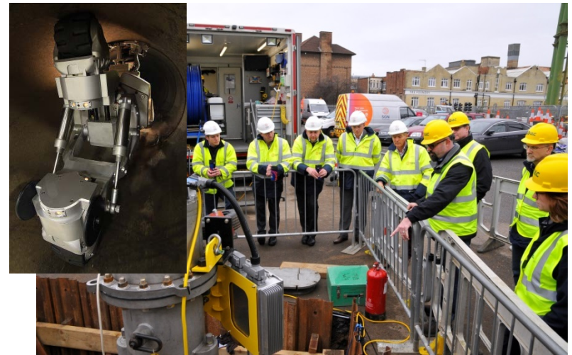
The CIRRIS XI™ and CIRRIS XR™ Robotic System for Large Diameter Cast Iron Gas Main, UK gas network, SGN and ULC Robotics, Inc.
