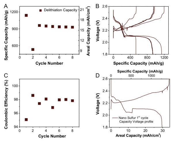
Fig. 4. Electrochemical performance of carrageenan based micro- and nano-sulfur electrodes. (A, B) Reversible capacity of 17.0 mg/cm<sup>2</sup> micro-sulfur mass loading electrodes based on carrageenan at 0.01 C. (C) Coulombic efficiency of the carrageenan based micro-sulfur electrode. (D) The initial capacity voltage profile of carrageenan based nano-sulfur electrode with the sulfur mass loading of 24.6 mg/cm<sup>2</sup>.
