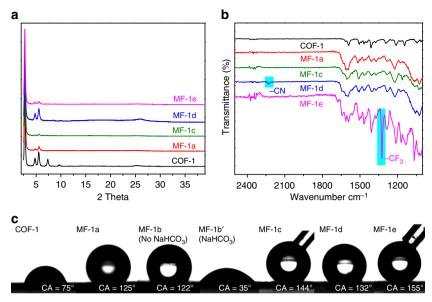
**Fig. 5** Structural characterization and surface properties of MF-1 series. **a** Powder XRD patterns of COF-1 (black), MF-1a (red), MF-1c (green), MF-1d (blue), and MF-1-e (purple). **b** FT-IR spectra of COF-1 and MF-1a, c-e. The peaks highlighted in cyan are characteristic vibrations from these functional groups. **c** Water contact angles (CA) of water droplet on the pressed pellet of COF-1 and MF-1a-e. MF-1b' is the NaHCO<sub>3</sub>-treated MF-1b that undergoes partial ester hydrolysis
