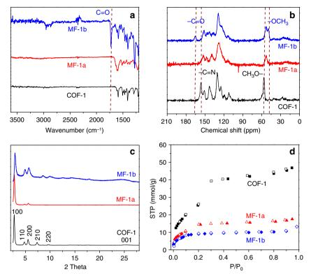
Fig. 2 Characterization of original COF-1 (black) and post-synthetically modified MF-1a (red) and MF-1b(blue). a FT-IR spectra. b Solid-state <sup>13</sup>C CP-MAS NMR spectra. c PXRD patterns showing retention of crystallinity after the Povarov reaction. d N<sub>2</sub> sorption isotherm curves
