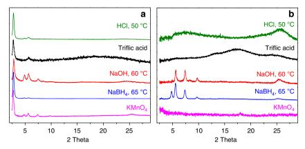
**Fig. 4** Chemical stability of MF-1a and COF-1. PXRD patterns of MF-1a (**a**) and COF-1 (**b**) after treatment with 12 M HCl at 50 °C for 8 h (green), 98% triflic acid at ambient temperature for 3 days (black), 14 M NaOH in  $H_2O/MeOH$  solution at 60 °C for 1 day (red), 5 equiv. of NaBH<sub>4</sub> in MeOH at 65 °C for 1 day (blue), and 5 equiv. of KMnO<sub>4</sub> in  $H_2O/CH_3CN$  solution at ambient temperature for 1 day (purple)
