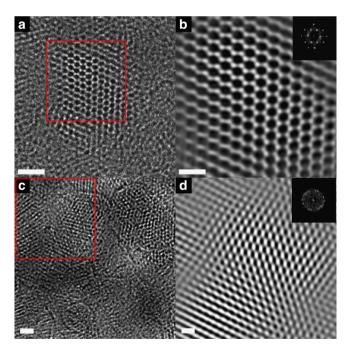
**Fig. 3** HRTEM characterization of COF-1 and MF-1a. **a** Low-dose, high-resolution TEM image of COF-1 (scale bar, 10 nm). **b** The Fourier-filtered image of selected red square areas (scale bar, 5 nm), Inset: Fast Fourier Transform (FFT) from the red square on the COF-1. **c** Low-dose, high-resolution TEM image of MF-1a (scale bar, 10 nm). **d** The Fourier-filtered image of the selected red square area (scale bar, 5 nm), Inset: FFT from the red square on the MF-1a
